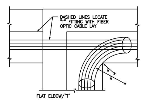
BENDING RADIUS FOR FIBER OPTIC CABLES AND CAT 6 AS PER MANUFACTURER'S SPECIFICATIONS AND TIA/EIA STANDARDS
