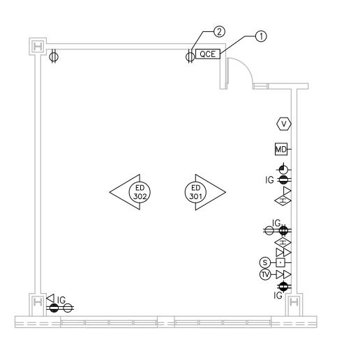
① CLASSROOM CONCENTRATOR SHOWN. ENGINEER OF RECORD TO LAYOUT ALL CONCENTRATOR ENCLOSURES ON FLOOR PLANS.
